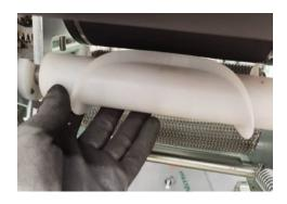
Place the cutter on the base and verify that it 3 is correctly installed and secured
