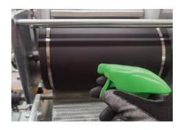
Spray grooves and straps with water to remove excess product
